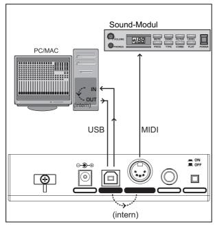
Fig. 2.1: Block diagram of MIDI signal flow
